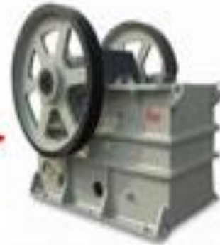
[2] Jaw Crusher Primary Crushing
